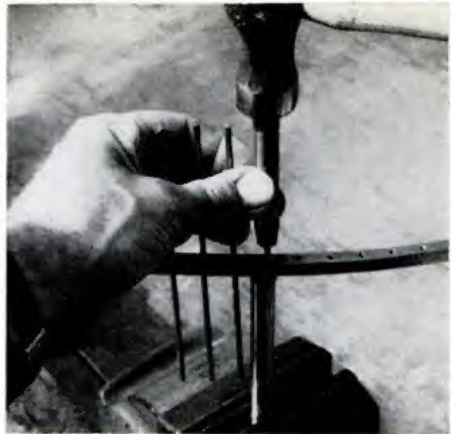
RIBS are driven with special setting tool. After all ribs are in place, cut them to the shape of a fish
